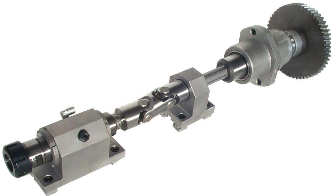
This attachment is designed to create polygons or geometrical profiles inside the component. It has to be fitted on the centre block of the machine (longitudinal slide).
