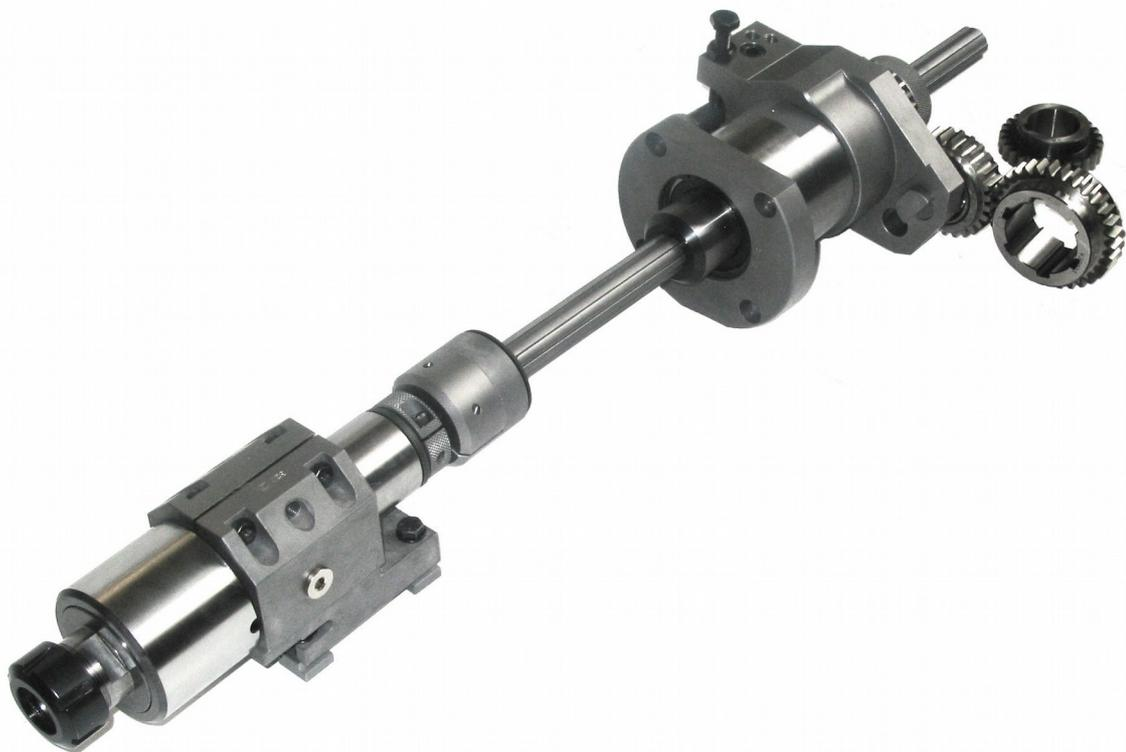
The High Speed Drilling Attachment rotates in the opposite direction than the bar, that allows to drill at higher cutting speed.
