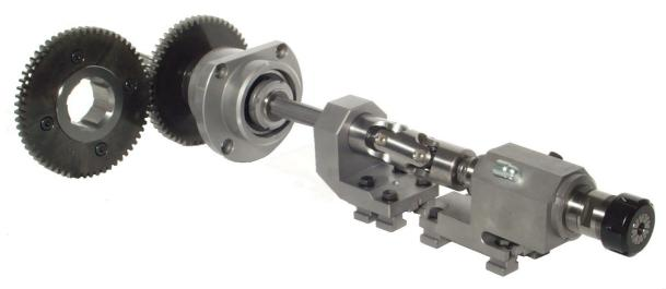
This attachment is designed to make polygons or geometrical profiles inside or outside the component, provided that they can be reached frontally.
