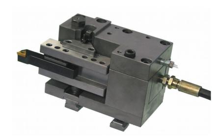
It has to be fixed on machine cross-slide. It can do part facing by X-movement of the cross slide.
