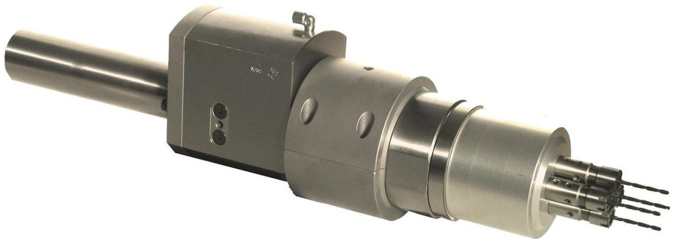
This multi-driller in particular is designed to make 4 drilled holes on a specific interaxis, we can supply it for a special spindle-stopping machine, but also for standard machines.
