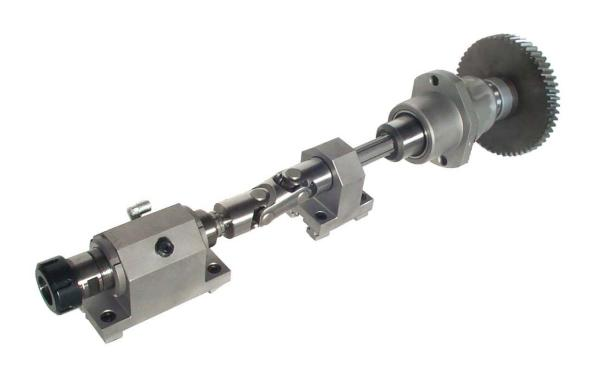
This attachment is designed to create polygons or geometrical profiles inside the component. It has to be fitted on the centre block of the machine (longitudinal slide).
